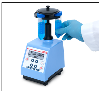
5. Check if tubes are firmly clamped
