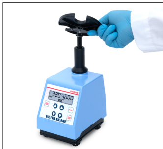
2. Put tube holder onto shaft
