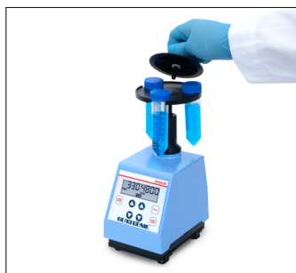
4. Put lid on and tighten thumbscrew
