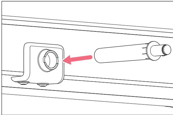
1. Insert the longer and thicker part of the door damper into the holder.
