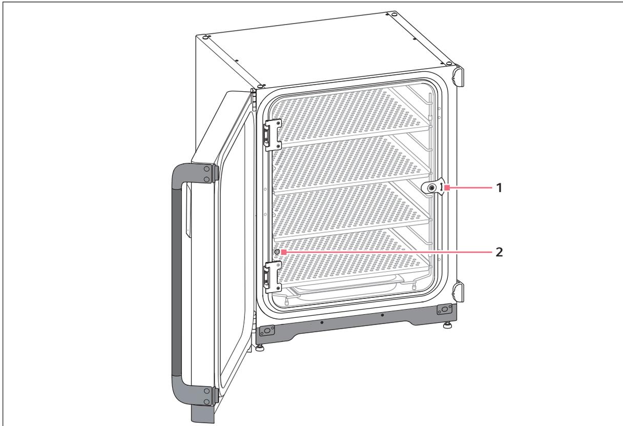
Fig. 3-5: Non-segmented inner door
