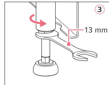
1. Loosen the lock nut with the supplied wrench of 13 mm.
