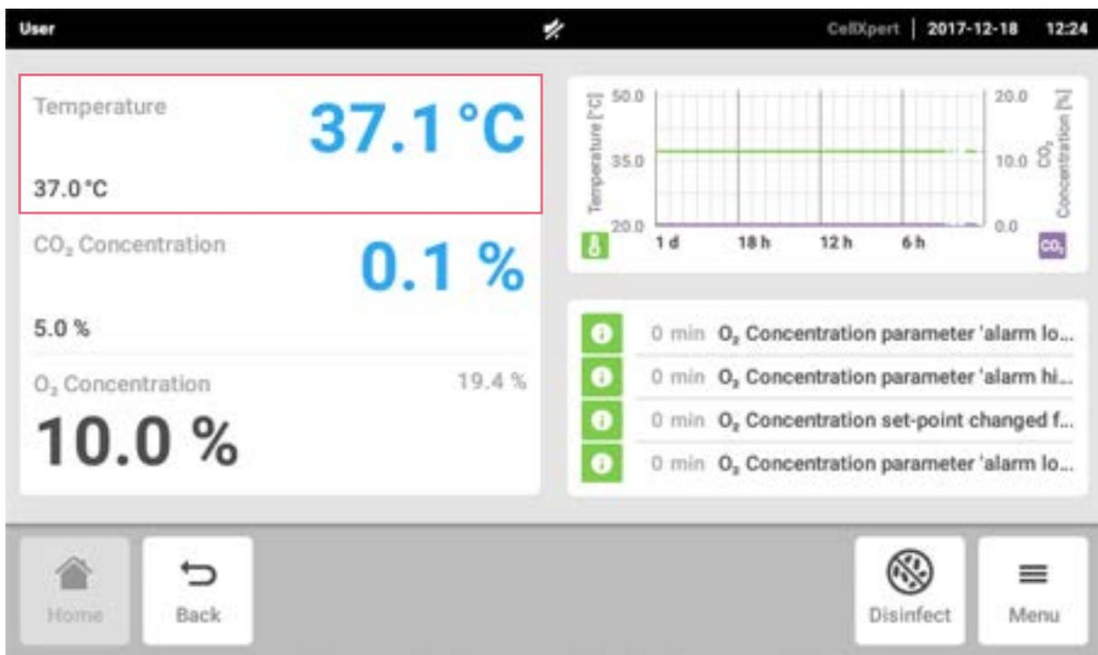
Tap the *Temperature* function in the function area. The parameter settings are displayed.
