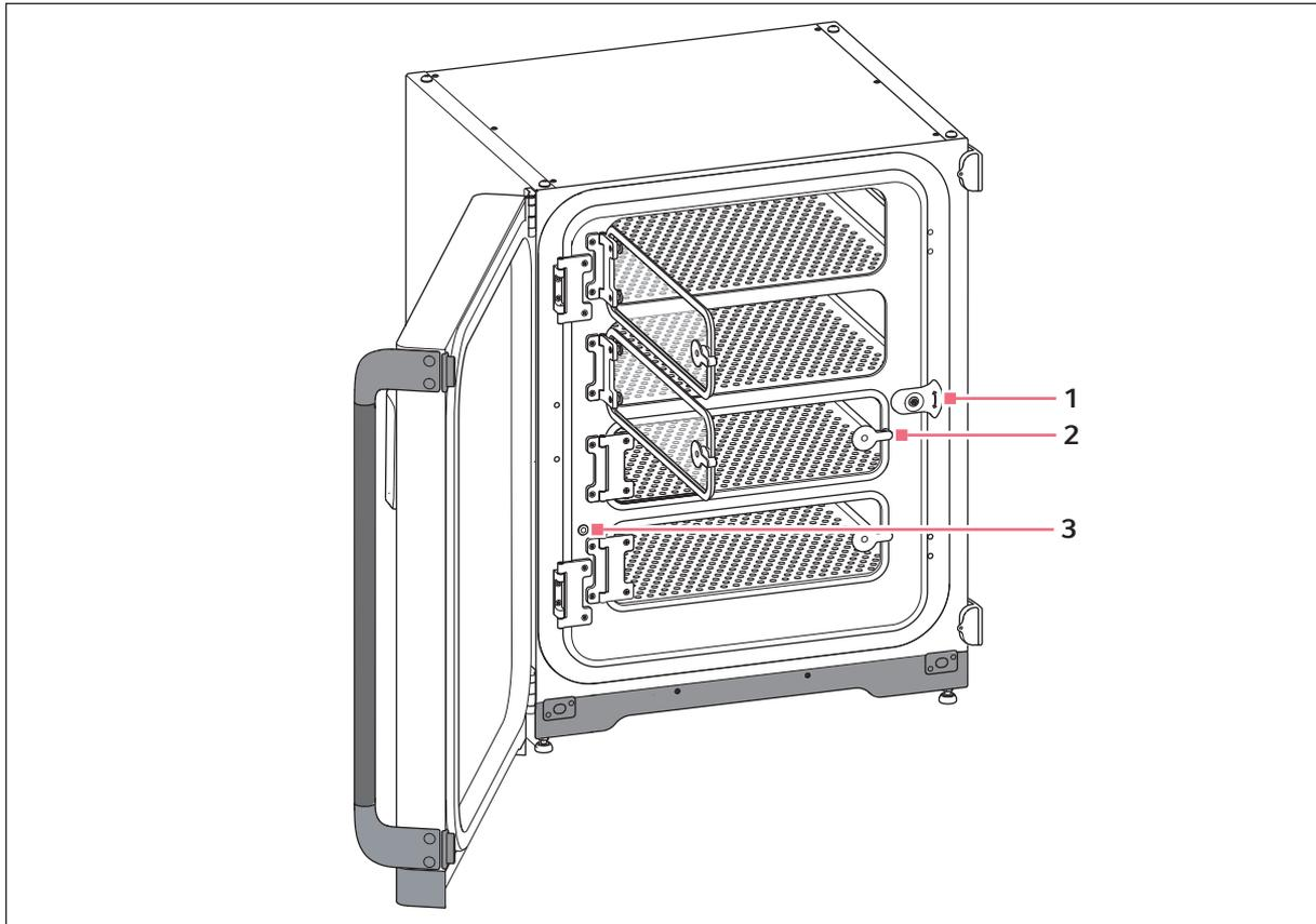
Fig. 3-6: Inner door with 4 door segments
