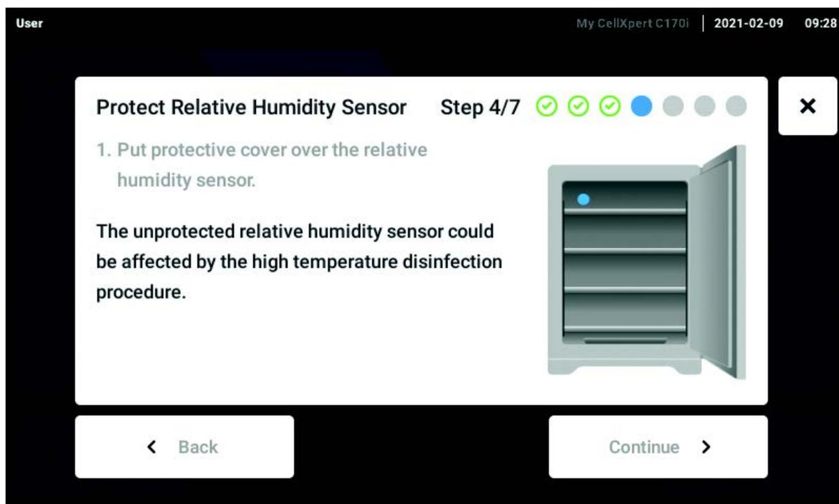
Put the protective cover up on the humidity sensor and tap the button *Continue*.
