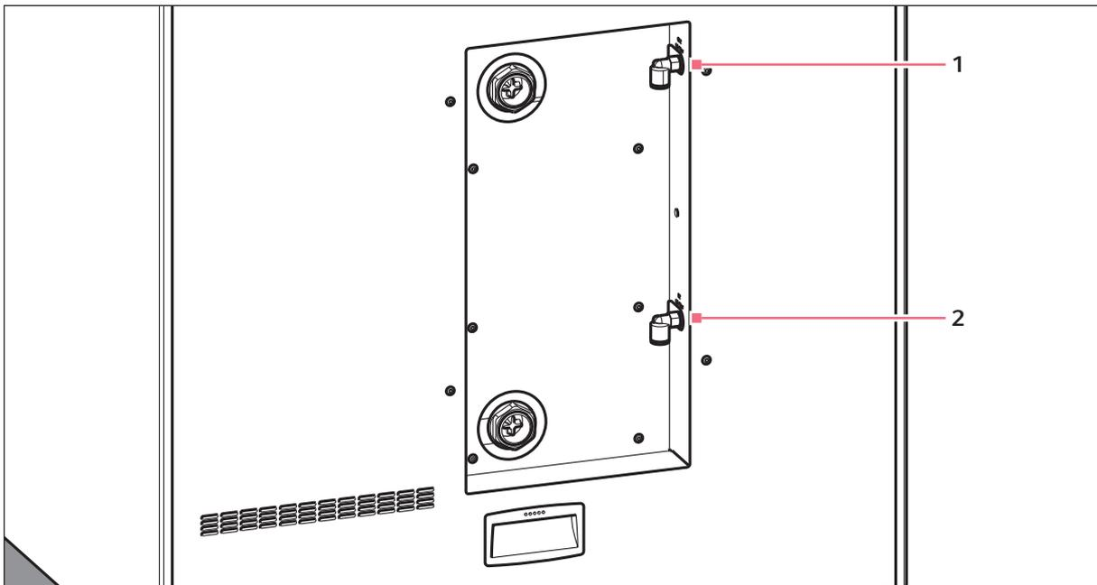
Fig. 4-1: Connections for CO<sub>2</sub> and N<sub>2</sub> at the rear of CellXpert C170i
