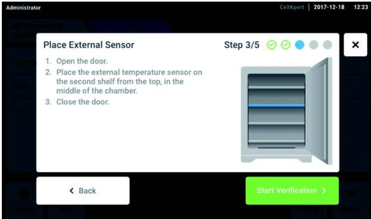
Fig. 10-3: Placement of the external temperature sensor
