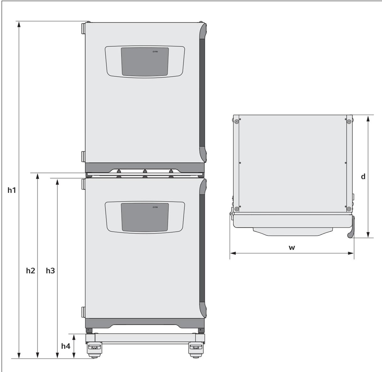
Fig. 13-2: Dimensions of 2 stacked CellXpert C170i (without safety latch)
