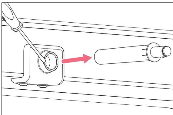
1. Remove the door damper with the flat head screwdriver.
