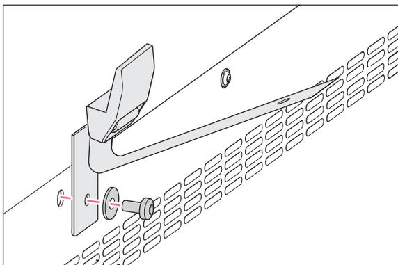
2. To attach the lower part of the safety latch to the top side of the incubator, use the spare part screw M4x8, Torx 20, and a washer.
