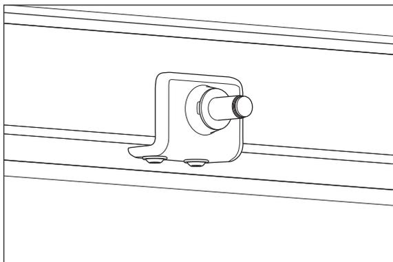
2. Press the door damper into the holder until it stops.
