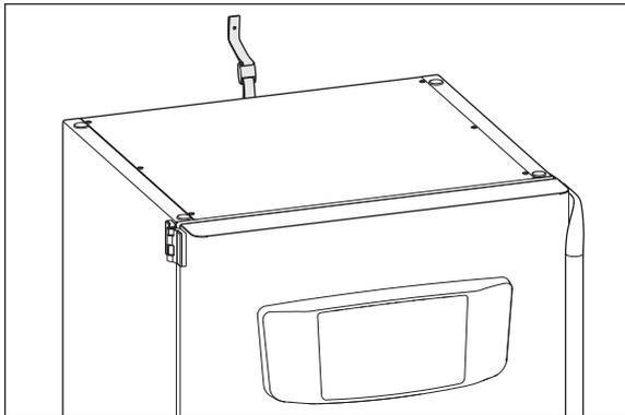
4. Click the two parts of the magnetic safety latch together.
