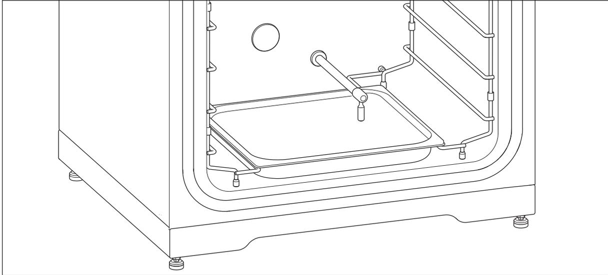
The water level sensor is located above the water tray. The flexible end of the water level sensor allows the user to remove and insert the water tray easily.
