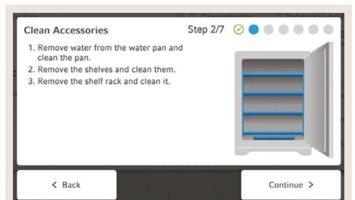
**Figure 2:** Modern CO<sub>2</sub> incubators can have clear step-by-step instructions for standardized cleaning procedures to be carried out before sterilization at 180 °C. To further reduce the probability of user errors the process should be sensor supported.
