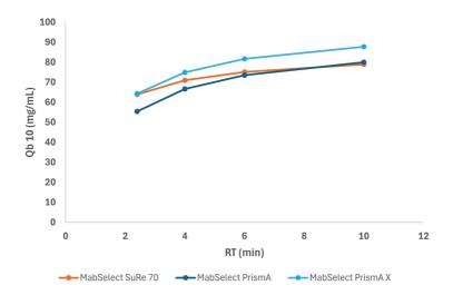
As MabSelect PrismA X has high dynamic binding at short residence times, the resin is suitable to use in rapid cycling chromatography (RCC) mode to further reduce resin volumes, increase grams of mAb produced per liter of resin, and decrease overall resin costs.
