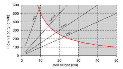
Choose a residence time that meets the requirements for dynamic binding capacity and fluid velocity according to the figure above. The other cycle operations including wash, elute, and equilibration steps can be run at maximum operational flow velocity, see *Resin properties, on page 5*.
