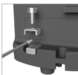
Connect the scale to the equipotential bonding conductor using an equipotential bonding cable with a gauge of at least 4 mm<sup>2</sup>.
