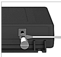
Connect the ex-link converter to the equipotential bonding conductor using another equipotential bonding cable with a gauge of at least 4 mm<sup>2</sup>.
