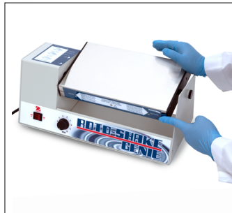
5. For rocking, press Release button, align Pin Slot on Platform with Pin on housing and shift Platform to the left, then let go of the Release button
