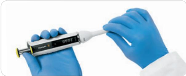
1. Unscrew the tip ejector collar counter clockwise and remove it. Remove the Safe-Cone Filter if fitted.
