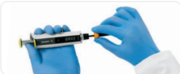
2. Unscrew the tip cone holder counter clockwise and carefully remove it along with the tip cone.
