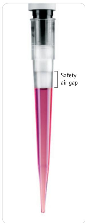
SafetySpace Filter Tips, made of virgin polypropylene, feature filter barriers that effectively capture solid and liquid aerosol particles. The filter is made of polyethylene without self-sealing additives to avoid any interference with the sample and results. The filter protects the sample against contamination. In addition, it protects the pipette and prolongs the maintenance interval of the pipette.
