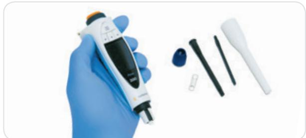
5. After performing the procedure described above, remove the components from the beaker and rinse them with distilled water, then dry preferably in warm air, for at least an hour.
