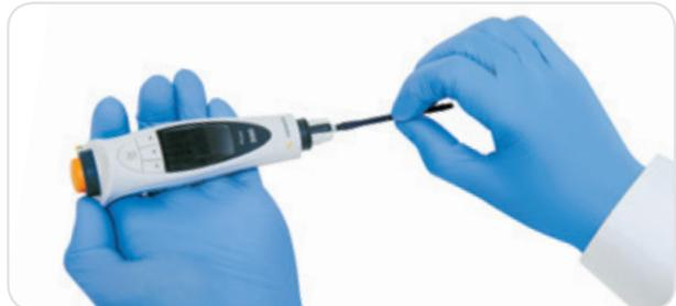
3. Unscrew the piston counter clockwise from the pipette.
