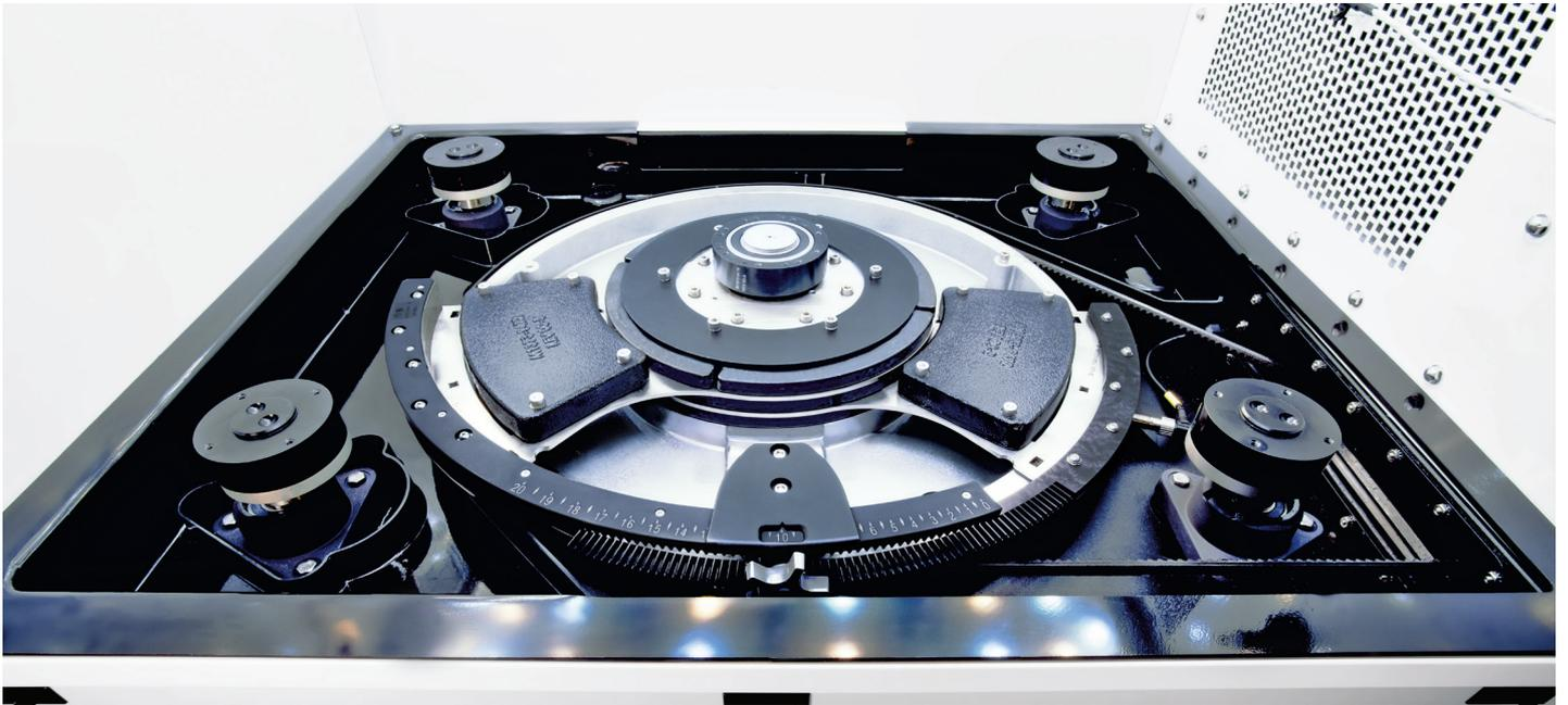
Shake faster, smoother, and longer with the new Eppendorf X-Drive Shaker Mechanism. The five eccentric mounting points for the shaker platform are precisely engineered to ensure long-lasting, repeatable performance for years to come. The four shafts in the corners and Balance Master Technology support precise vibration-free shaking on every point of the platform, including the periphery. Available in two orbit sizes: 2.5 and 5.1 cm (1 and 2 in).
