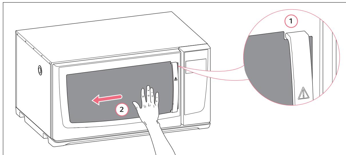
**1 Cut-out of the window shade****Auxiliary equipment**
