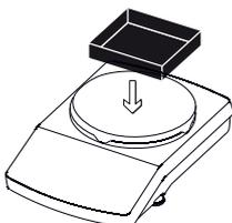
▶ Place the container for the first component on the weighing pan.
