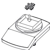
▶ Remove the first component from the weighing pan and place the next component on the balance.
