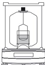
▶ Place the sample on the weighing pan above on the frame of the density determination kit.
