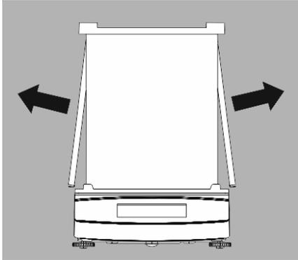
7) Pull out the draft shield frame from the side of the guide
