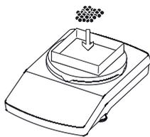
▶ Place the first component on the weighing pan.
