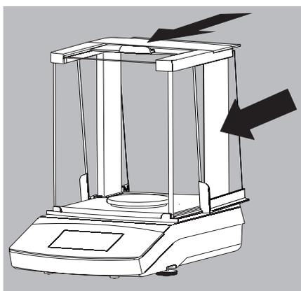
2) Push the three glass panels into the draft shield guide, all the way to the front.
