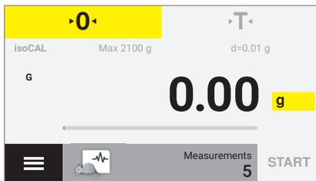
▶ The **Unstable condition** application appears. The set number of measurements is displayed under **Measurements**.
