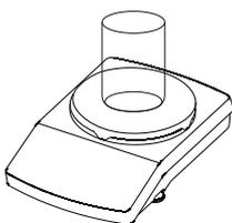
▶ Place a container on the weighing pan.
