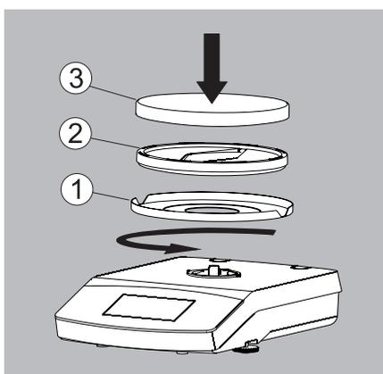
3) Install the pan support (1) and weighing pan (2).
