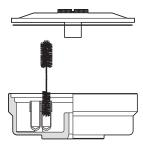
Wash rotor components immediately if salts or other corrosive materials are used or if spillage has occurred. Do not allow corrosive materials to dry on the rotor.
