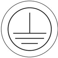
This symbol is used to indicate a protective ground. This instrument must be properly grounded. Do not under any circumstances operate the instrument unless it is properly grounded.
