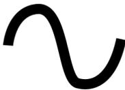
This symbol is used to indicate an alternating current (also known as “AC”).
