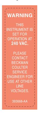
This symbol indicates that the instrument has been configured for operation at 240 VAC. Consult with a Beckman Coulter service engineer for use at other line voltages.
