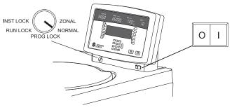
The power switch is a two-position rocker switch (I, on; O, off) which controls electrical power to the centrifuge.
