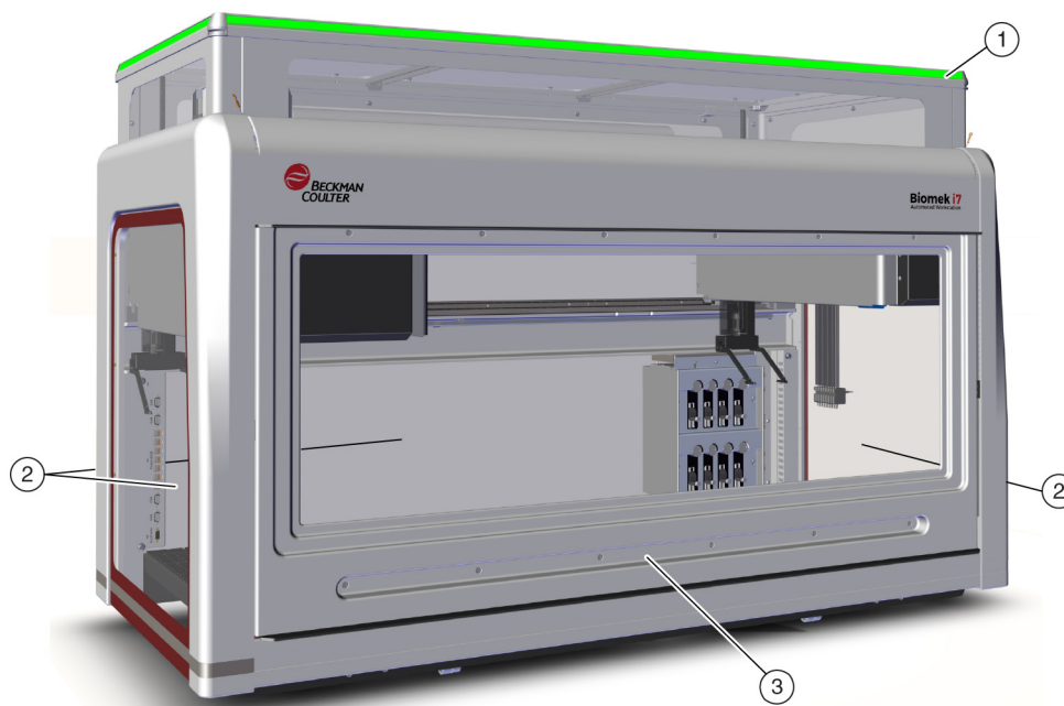
Figure 1.11 Protective Barriers for an Enclosed Biomek i-Series Instrument
