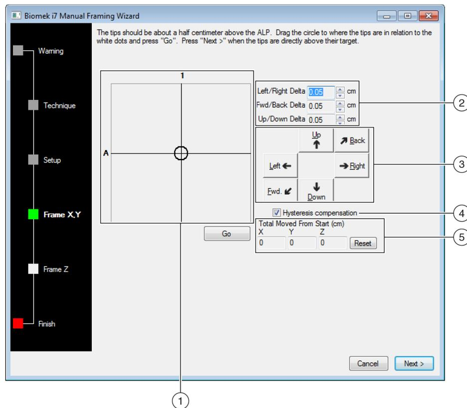
1. **Graphic Alignment Tool:** The graphic alignment tool is a visual representation of the tip (small circle) and the framing points (large circle). The small circle is moved until it represents the tips position in relation to the framing points on the ALP.
