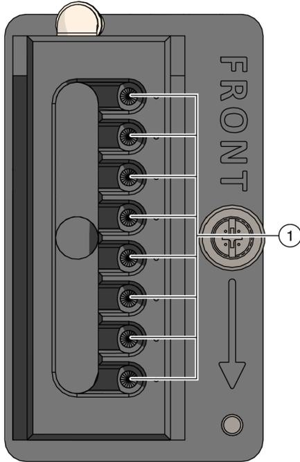
1. **Framing Targets:** Align the tips to these small white dots on the ALP.
