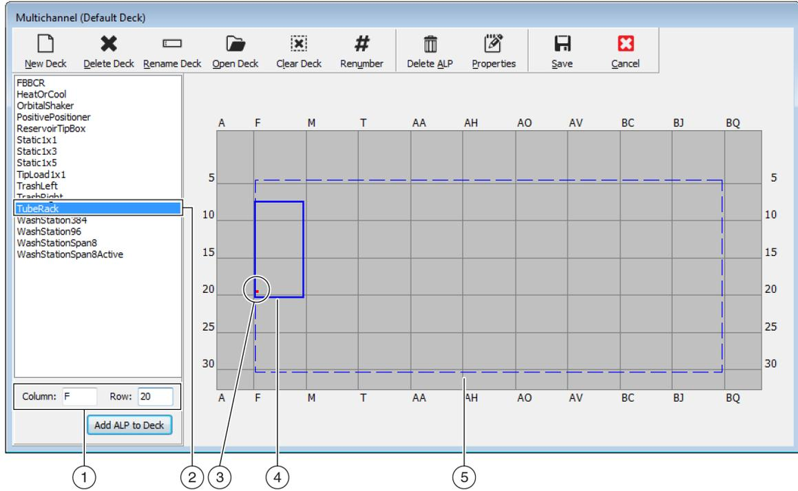
1. **Column and Row fields:** The location of the pointing feature when the ALP is physically installed on the deck.
