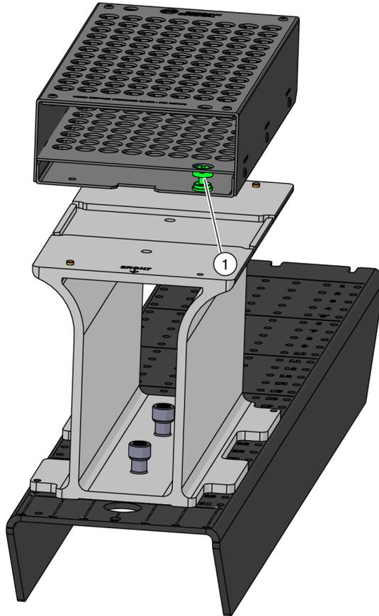
1. Labware-Positioning Screw (back-left screw not shown)
