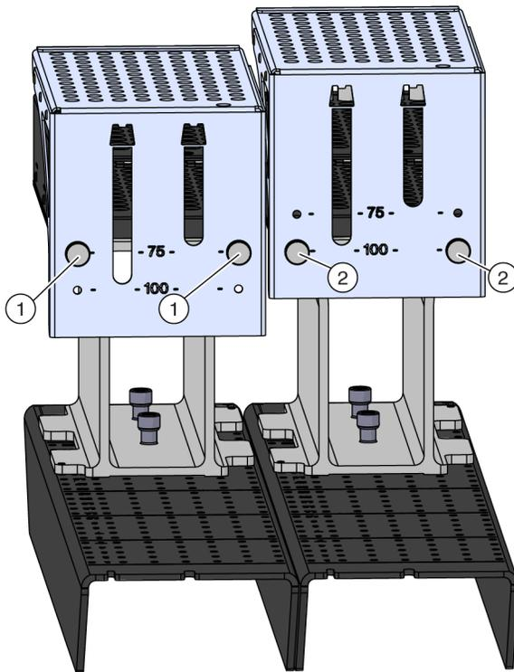
1. Thumbscrew locations for test tube racks containing 75 mm test tubes.
