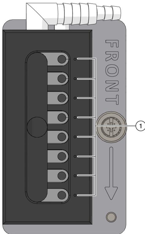
1. **Framing Targets:** Align the tips to these small white dots on the ALP.
