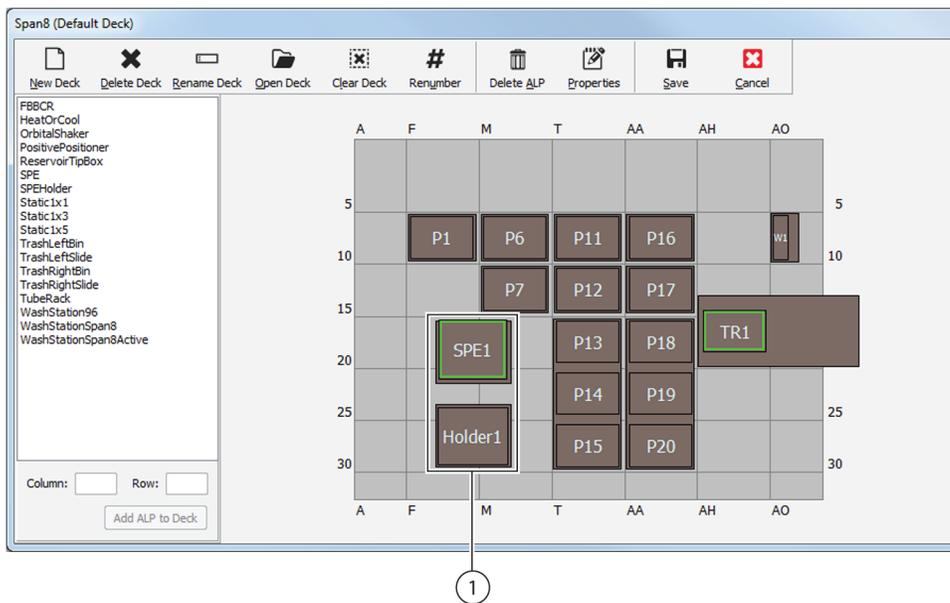
1. First frame the SPE ALP, then use that framed position as a reference point to frame the SPE Collar Stand
