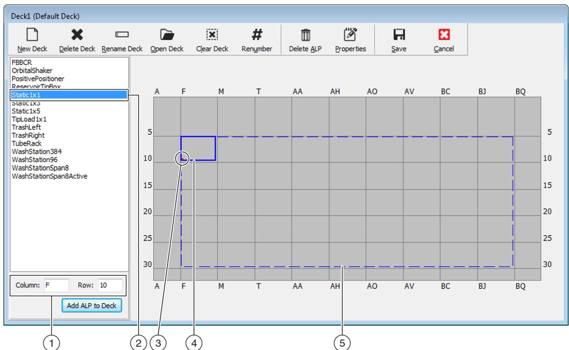
1. **Column** and **Row** fields: The location of the mounting point when the ALP is physically installed on the deck.
