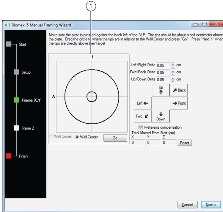
1. The graphic alignment tool is a visual representation of the tips (small circle) and the well of the labware (large circle) at the position being framed. The small circle is moved until it represents the tips' current physical location in relation to the well of the labware.
