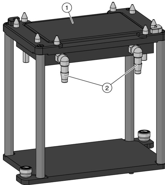
1. Heating & Cooling unit: Mounted to an ALP stand.
