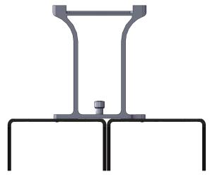
The deck plates can be fastened directly to the chassis with screws using the hole located in the front of the deck plate, and the slot at the back (Figure 13).
