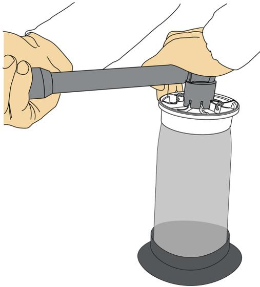
To aid in achieving the proper torque, [Contact Us](#) to order the bottle grip (PN 366763). Pushing down on the bottle can help prevent the bottle from slipping in the grip. Make sure when pushing down that you are not pushing on the cap, as this could prevent the cap from receiving the full torque.
