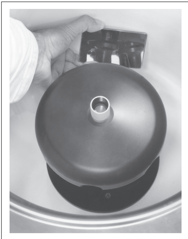
Figure 5.8 Checking Hook-on Bucket Positions After the Rotor is Installed*
