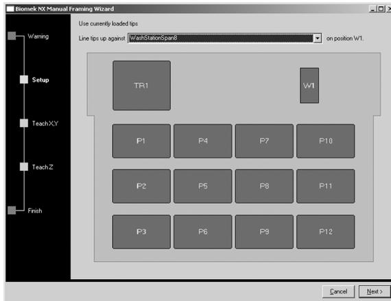
**7** If no tips are loaded, in **Load tips from the**, select the type of tips to load and the **position** on which the tip box is located (Figure 2.11).
