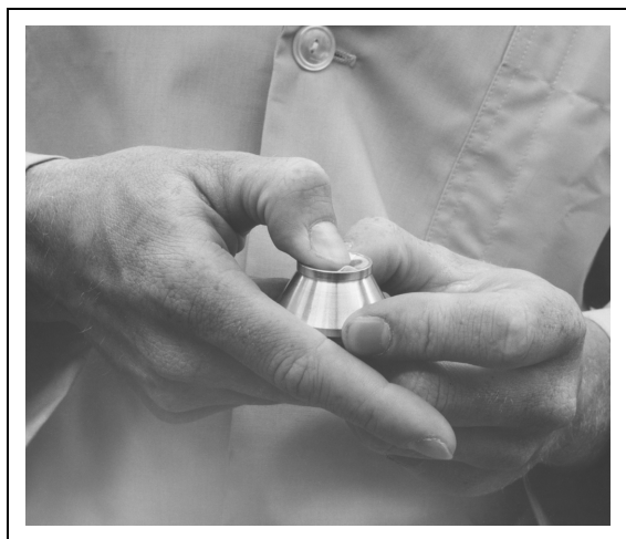
Figure 4. Removing the Rotor Cap. Press in the center of the cap to free an edge.
